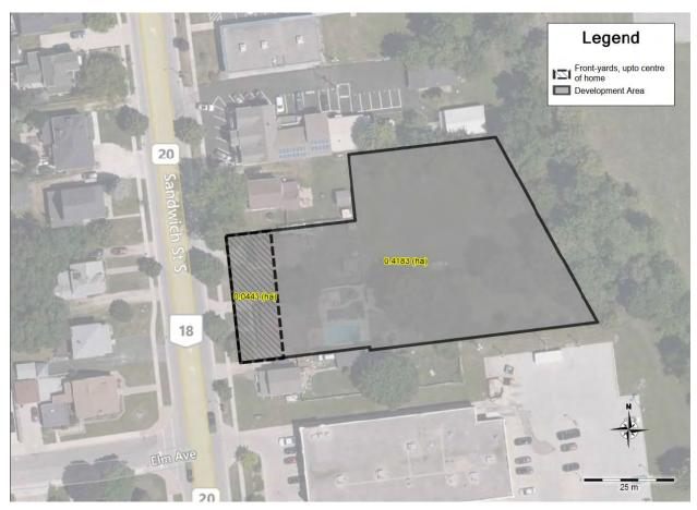
FIGURE 1: EXISTING CONDITIONS ANALYSIS DRAINAGE AREA COMPARED TO TOTAL DEVELOPMENT AREA
