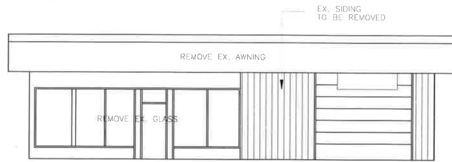
EXISTING NORTH ELEVATION
