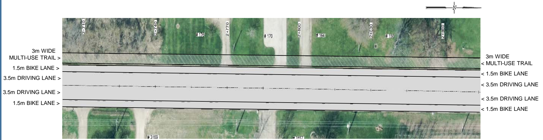
Typical Plan View of Proposed Design III – Simcoe Street to Alma Street
