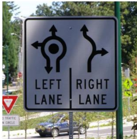
Multi-lane Roundabout Signage
