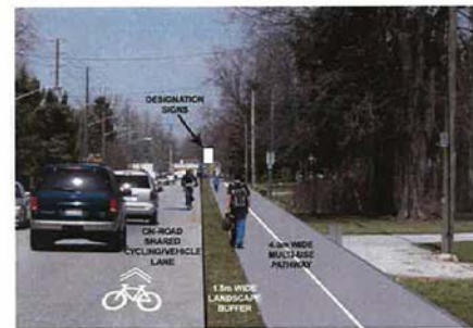
MALDEN ROAD - POSSIBLE ON-ROAD SHARED CYCLING/VEHICLE LANE
